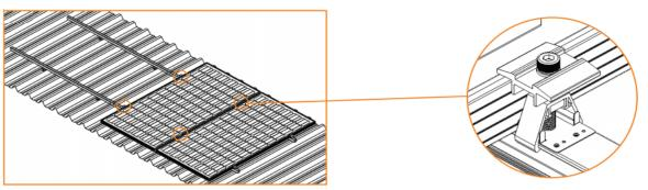
Put the second panel on the rail, fasten the mid clamps with inner hex bolts M8 at all locations where two panel meet  $\cdot$ .
