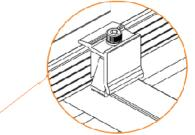
Install all the panels and tasten end clamps at the end of each array.
