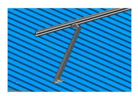
9.5 As the requirement of planning the array layout attach front leg & rear leg and rail on the roof.
