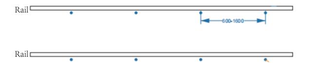
The Tilt kit hooks should be fixed to the rafter using 6.3x90mm wood screws minimum. Or use sellf tapping bolts to fix on steel purlin
