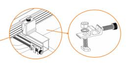
Install a grounding lug onto each rail line edge with an inner hex bolt M8\*25 and a stainless steel nut, then connect 8.4mm2
